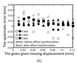
**Figure 1:** (a) the relationships between the systematic error and scanning time, (b) the relationships between the given moving displacement and the systematic error
