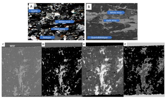
Figure 1. A) Optical and B) SEM images of the mylonitic metagranite (long side of the photograph = 1 mm). A sagittal section of the sample investigated by synchrotrn X-ray microtomography (isotropic voxel size = 9  $\mu$ m): C) as reconstructed, D) k-means clustering segmention of the image reported in D), E) after phase-retrieval and F) k-means clustering segmention of the image reported in E).
