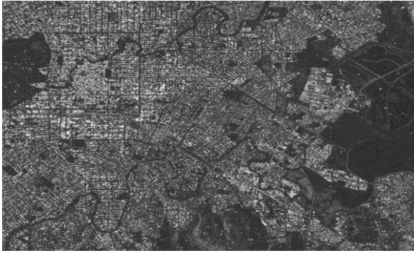
Figure 3. Average coherence image of Christchurch before the earthquake of 22 February 2011
