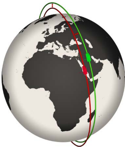
Figure 2. Orbit illustration of Helix formation. Red: TSX, Green: TDX; typical baseline values vary from 120 to 500 m.
