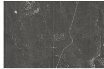
Figure 17. KOMPSAT-5 SAR image of the deployed CRs
