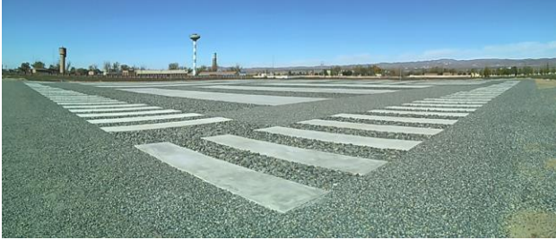
Figure 5. Bar-pattern permanent target
