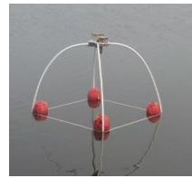
(h) Infrared water-leaving radiance measuring system
