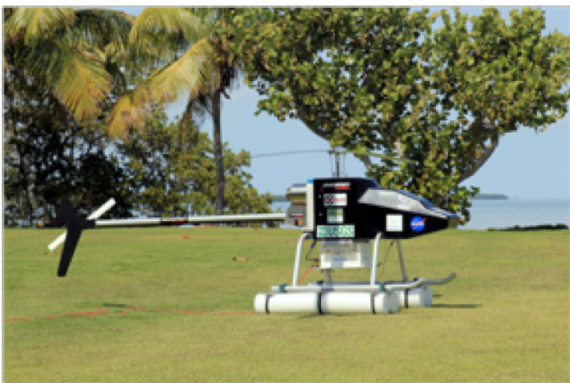
Figure 4. Vision-II UAS carrying NovaSol hyperspectral imager
