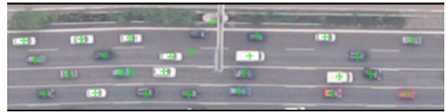
Figure 5: Car detection using adaboost image classification
