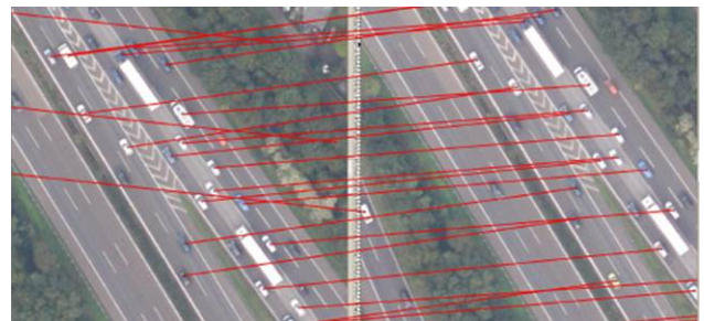
Figure 6: Tracking of cars using shape-based matching
