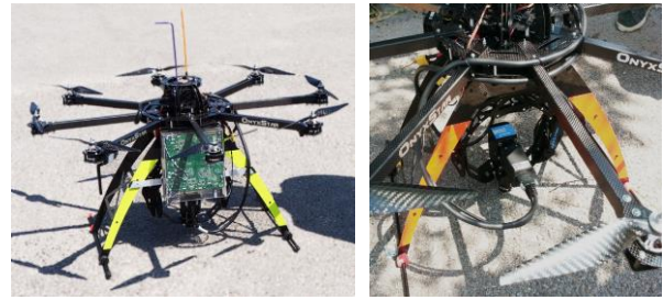
Figure 1. The multicopter equipped with the push-broom hyperspectral VNIR (380nm-1000nm) imaging sensor.
