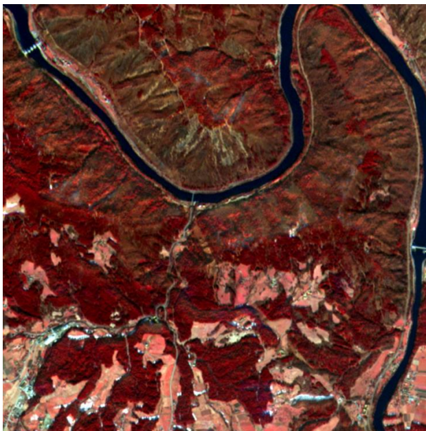
Figure 12. Comparison between false-colour composite image before (above) and after (below) the automatic topographic corrections (detail). On the corrected image the influence of topography is extensively reduced.
