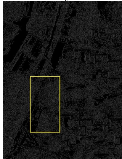
Figure 2. This figure shows the outline of image segmentation on the original image after converting the original image to greyscale. The area in the yellow box is part of road that is in the shadow. As it can be seen the vehicle in the shadow is not recognisable.
