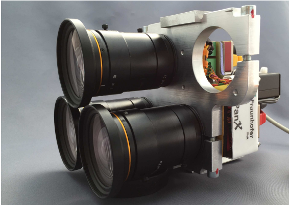
Figure 12. Three channel configuration of the PanX system for NDVI imaging.
