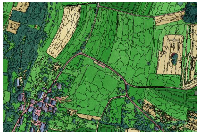
Figure 3: Fine-grained subdivision of the image after threshold-based and multiresolution segmentation (NATFLO)
