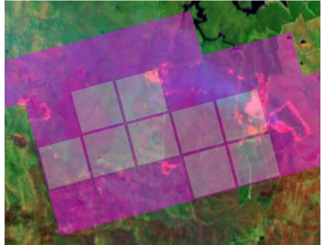
Figure 9. MODIS fire mask overlaid on the real-time Landsat image in the previous figure (dark pink: high confidence, light pink: nominal confidence fire pixel)
