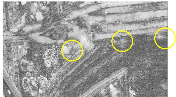
Figure 5. Disparity map using dynamic programming algorithm (Detect poles and power lines seems some extent and also the vegetation in white color).
