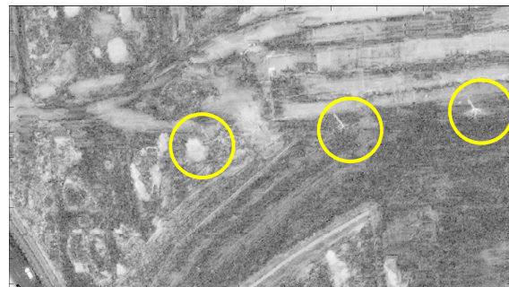
Figure 6. Disparity Map using Graph-Cut algorithm (Detect poles and power lines seems some extent and also the vegetation in white color, well smooth, less noise).
