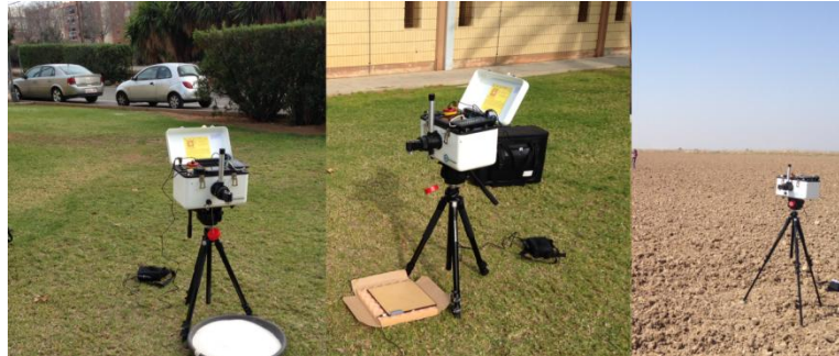
Figure 7. Mounting the spectroradiometer with sample White Sands (left), with the reflective panel (center) and the paddy soil sample (right).
