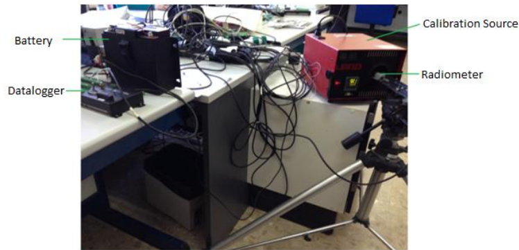
Figure 4. Experimental arrangement for calibration of the radiometer APOGEE SI-211
