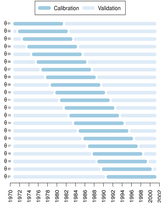
Figure 3: Illustration of the rolling calibration period methodology: 21 parameter sets \theta can be identified for each catchment.
